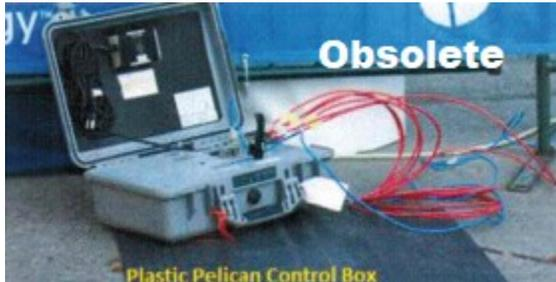
**Example 5:** If you see one of these, you know your side antenna won't work correctly. The long red cables shown will get in the way and degrade the RFID signal by 30%. The box is extra dead weight. Susceptible to rain. If Lithium Ion batteries are used they are prohibited on Airlines. Orbiter AGM batteries are approved for Airline travel. Lithium Ion is costly with surprise cancellation of airline tickets.
