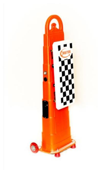
Auto connect with distributed database operating on a FIFO bases. Every tag read is EPOCH Time stamped at detection and held in non-volatile memory.
